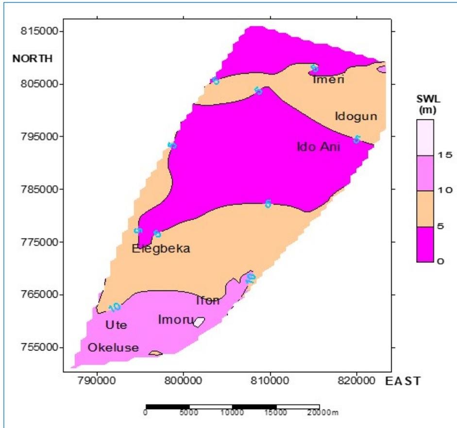
Fig. 6. Static water level map generated for the study area
