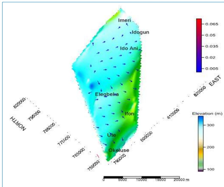
Fig. 2. 2-D Surface map overlay by 1-Grid Vector Map showing potential Groundwater flow direction
