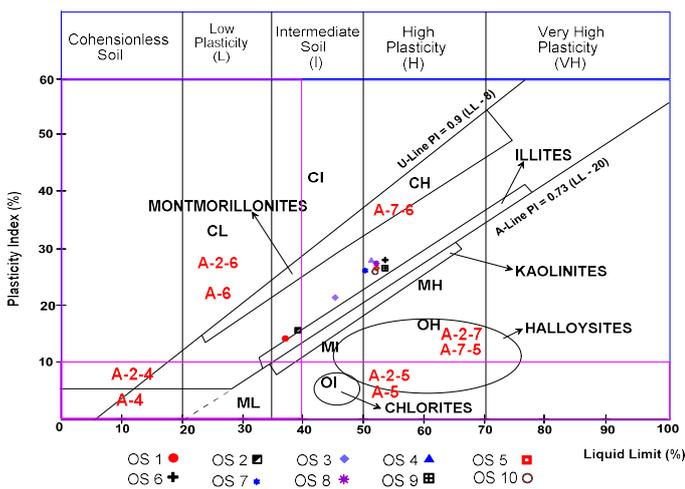
Fig. 8. Casagrande Plasticity Chart for the sampled soils showing predominantly High Plasticity
