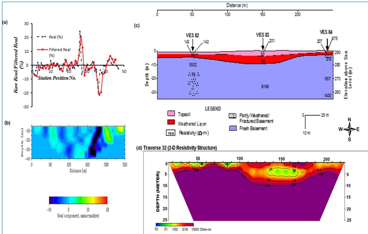
Fig. 12. (a) VLF-EM Real and Filtered Real Components, (b) VLF-EM 2-D Model, (c) Geoelectric Section, (d) Dipole-Dipole Resistivity Structure along Traverse 32 (Ifon-Ose)
