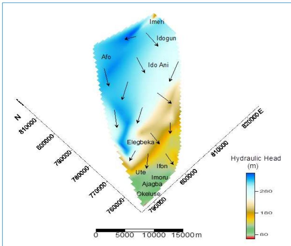
Fig. 7. Map of Hydraulic Head Measurements obtained in the study area
