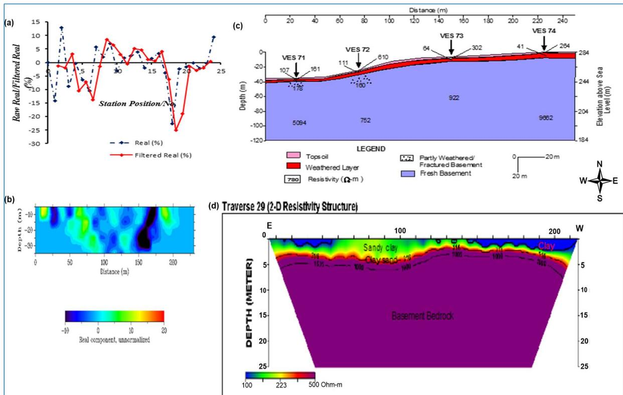
Fig. 11. (a) VLF-EM Real and Filtered Real Components, (b) VLF-EM 2-D Model, (c) Geoelectric Section, (d) Dipole-Dipole Resistivity Structure along Traverse 29 (Ido Ani-Ose)
