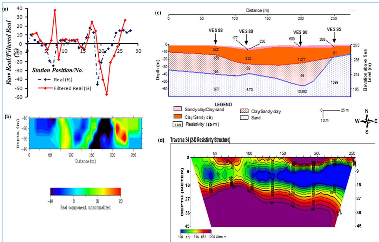
Fig. 13. (a) VLF-EM Real and Filtered Real Components, (b) VLF-EM 2-D Model, (c) Geoelectric Section, (d) Dipole-Dipole Resistivity Structure along Traverse 34 (Okeluse-Ose)
