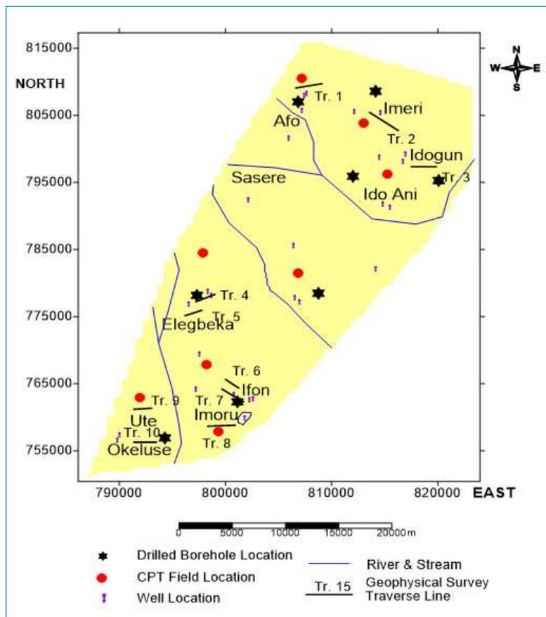
Fig. 5. Base map for geotechnical, geophysical, and borehole sampling
