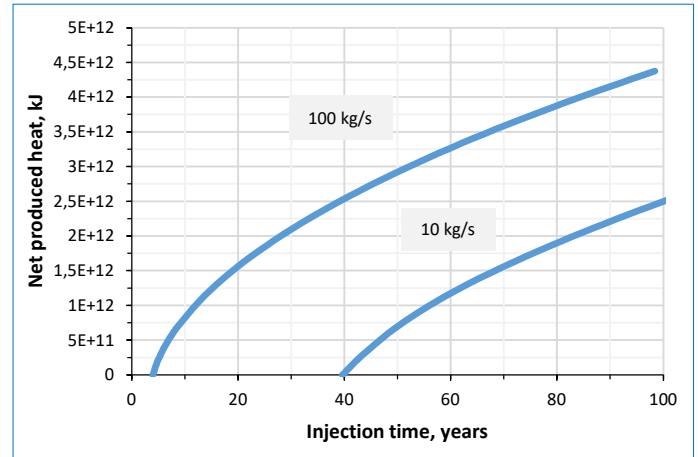
Fig. 9. Net cumulative production heat at the injection rates of 100 kg/s and 10 kg/s
