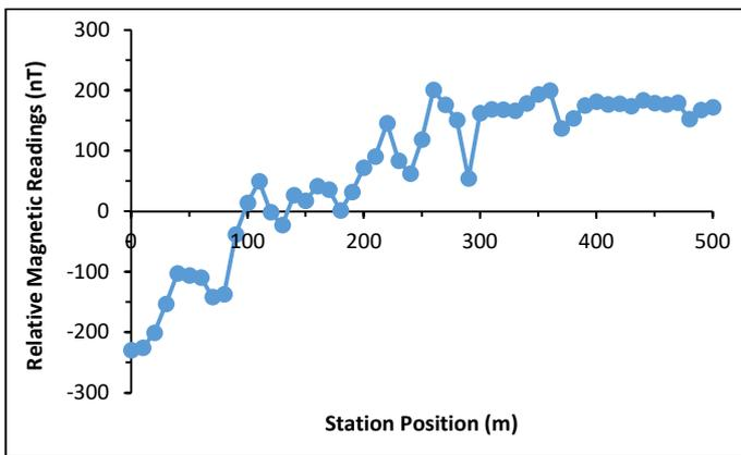
Fig. 5j. Magnetic survey profile (Korede profile)
