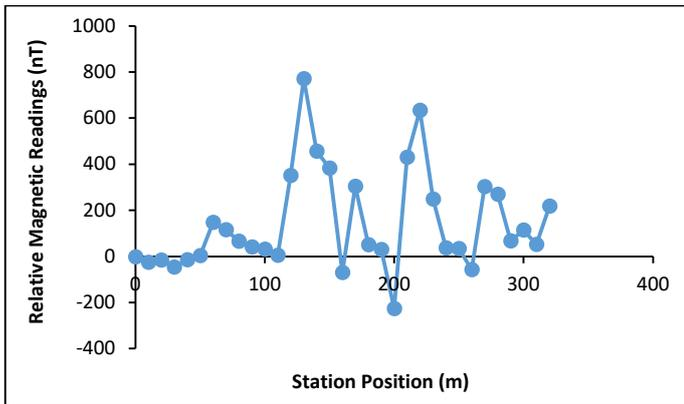
Fig. 5c. Magnetic survey profile (Sefari profile)
