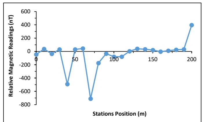
Fig. 5n. Magnetic survey profile (Yanmu Yanmu profile)
