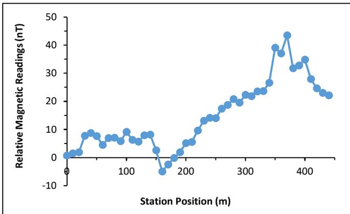
Fig. 5d. Magnetic survey profile (Okoru profile)
