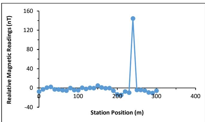
Fig. 5e. Magnetic survey profile (Alaaya profile)
