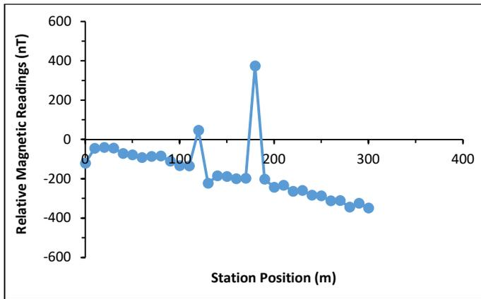
Fig. 5o. Magnetic survey profile (Yemoja profile)
