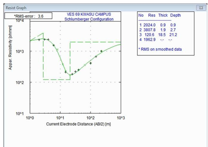
Fig. 6d. Typical HKH sounding curve
