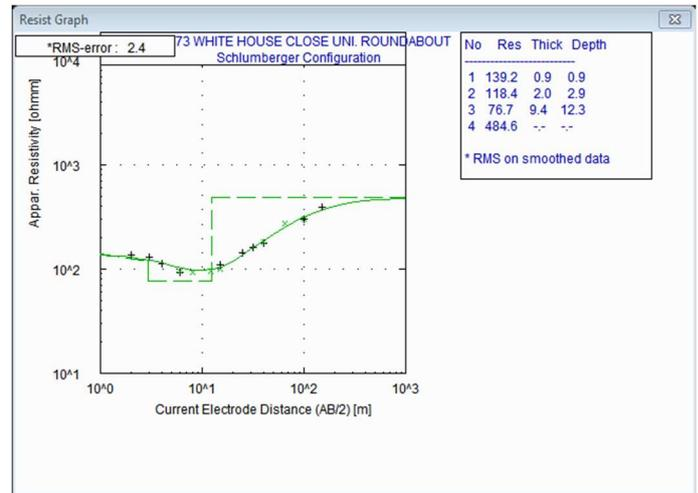
Fig. 6b. Typical HA sounding curve
