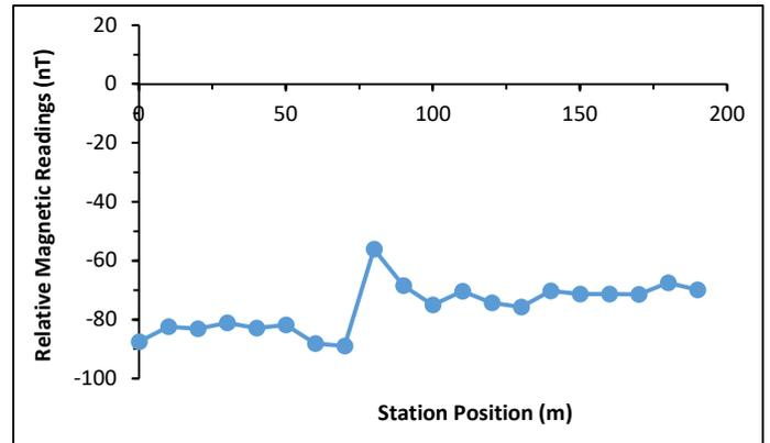
Fig. 5l. Magnetic survey profile (Alalubosa profile)
