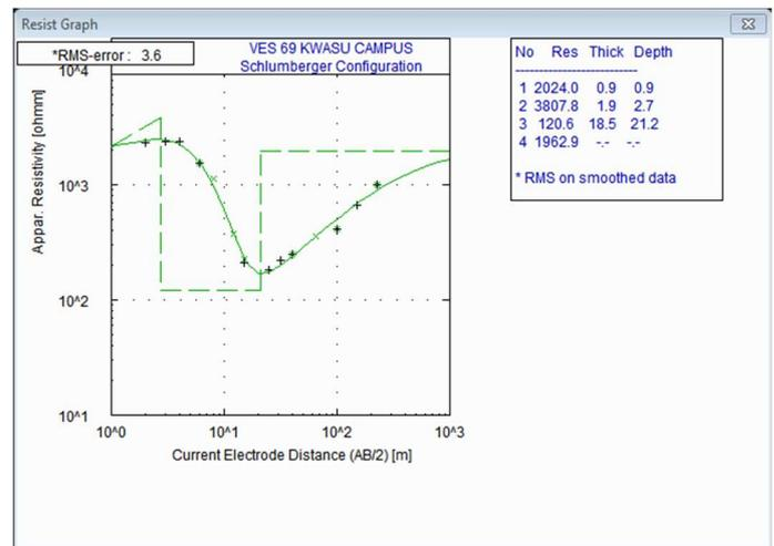
Fig. 6c. Typical kH sounding curve
