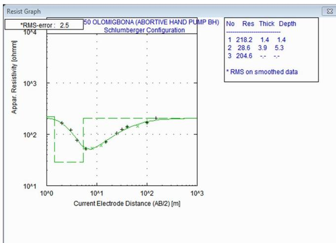
Fig. 6a. Typical H sounding curve
