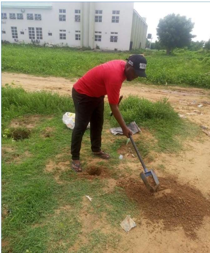
Fig.4. Soil sample collection using hand auger
