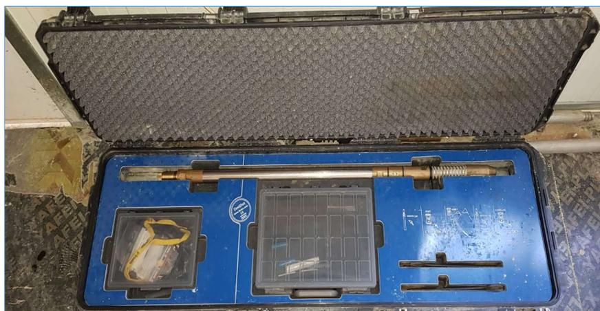
Fig. 5. Digital inclinometer device measuring borehole inclination
